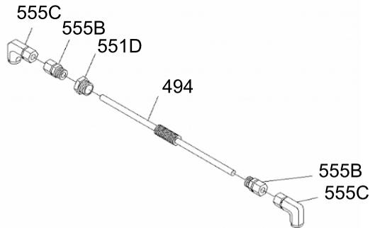
**Figure 143: Finned-tube oil cooler exploded view**
