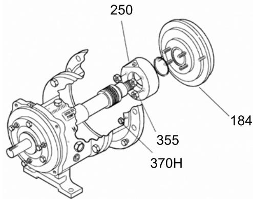
**Figure 72: Bearing housing and bearing removal**
