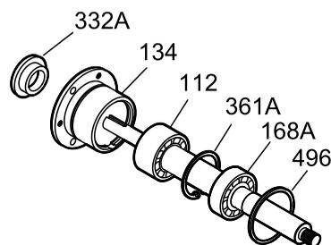
**Figure 97: Outboard labyrinth oil-seal reassembly**
