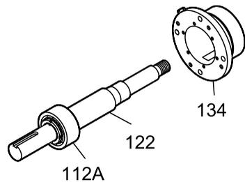
11. Remove the bearing locknut (136), the bearing lockwasher (382), and the outboard bearing (112A).
