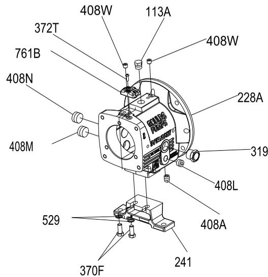
**Figure 137: Replace two grease fittings with two plugs**
