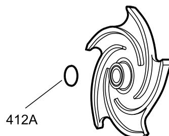
**Figure 56: O-ring for models 3196 and HT 3196**
