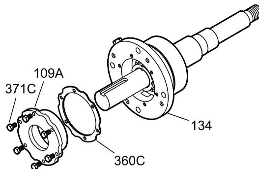
8. Install the inboard bearing as follows (see the illustration):
