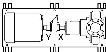
**Figure 30: Top view of an incorrect horizontal alignment**
