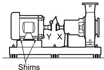
Figure 29: Side view of an incorrect vertical alignment
