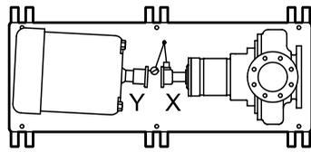
Figure 28: Top view of an incorrect horizontal alignment
