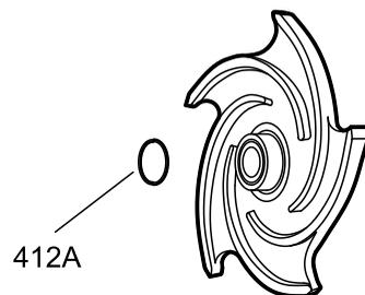
**Figure 55: O-ring for models 3196, HT 3196, NM 3196, 3198, and 3796**
