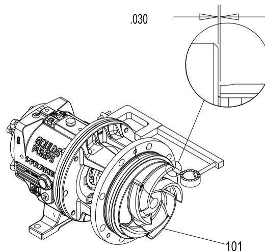
**Figure 131: Check impeller run out**
