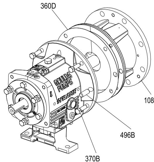
**Figure 114: Align bolt holes and dowel locations**
