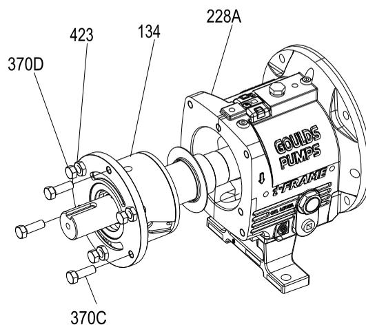
Figure 70: Shaft assembly removal
