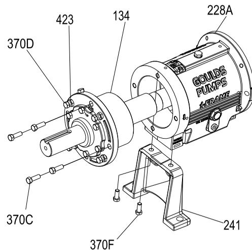
2. Remove the clamp screws (370C) and back off the jam nuts (423).
