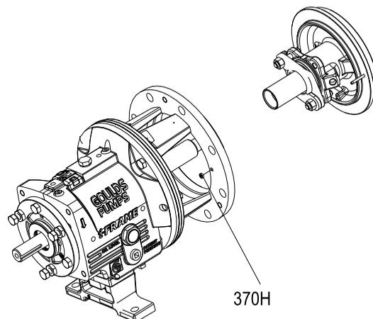
**Figure 119: Dynamic seal installation**
