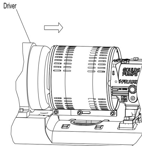
3. Remove the nut, bolt, and washers from the driver half of the coupling guard.
