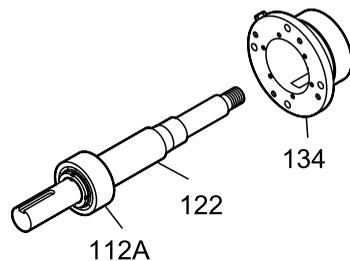
10. Remove the bearing locknut (136), the bearing lockwasher (382), and the outboard bearing (112A).
