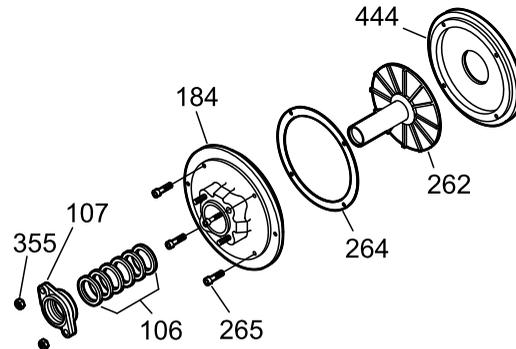
**Figure 118: Backplate placement**
