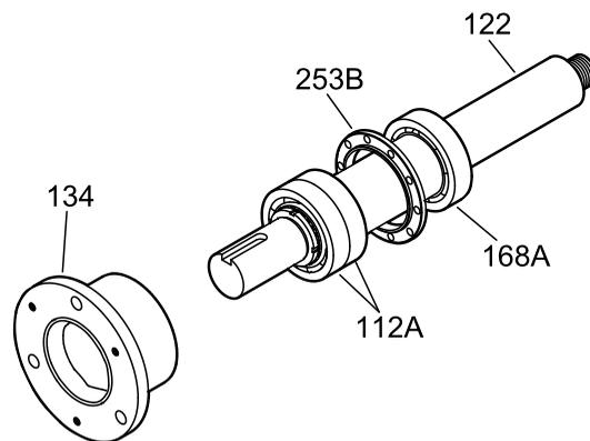
**Figure 102: Bearing housing reassembly**
