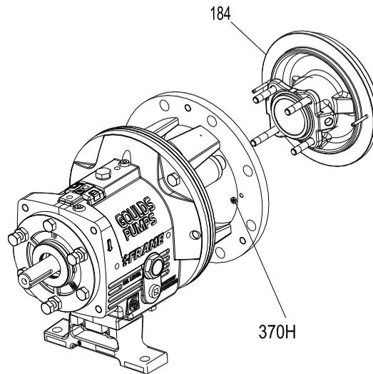
**Figure 123: Assemble seal-chamber**
