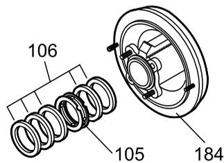
**Figure 61: Remove the shaft sleeve**
