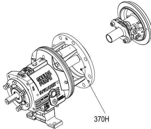
**Figure 63: Dynamic seal removal**
