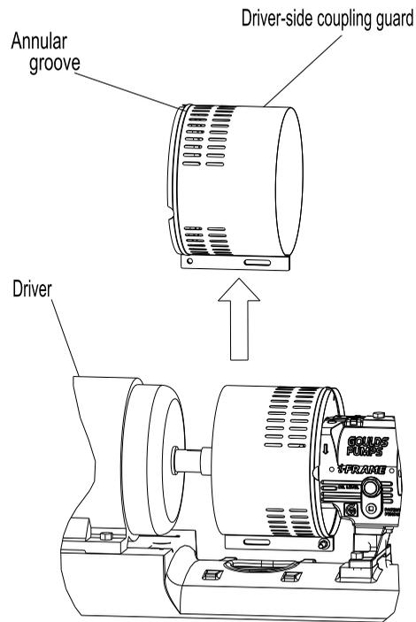
6. Remove the remaining nut, bolt, and washers from the pump half of the coupling guard. It is not necessary to remove the end plate from the pump side of the bearing housing. You can access the bearing-housing tap bolts without removing this end plate if maintenance of internal pump parts is necessary.
