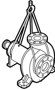
**Figure 1: Example of a proper lifting method**
