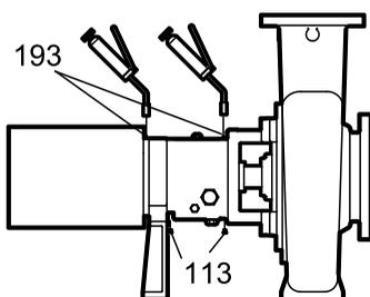
**Figure 49: Bearing lubrication**
