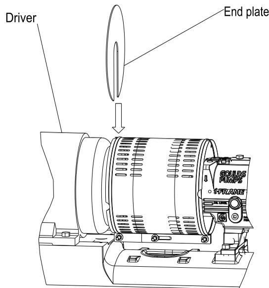
**Figure 42: Placement of driver half of coupling guard**
