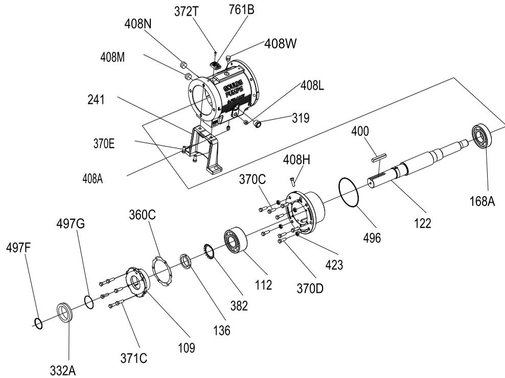
**Figure 142: XLT-i bearing-frame exploded view**
