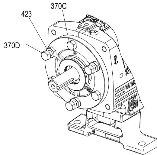
**Figure 133: Loosen clamp bolts and jack bolts on bearing housing**
