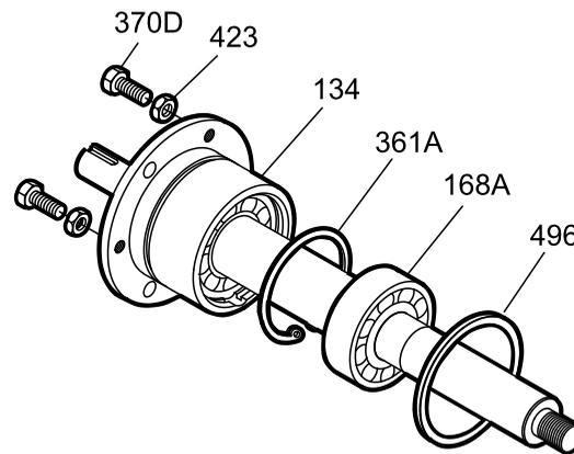
**Figure 67: Outboard bearing retaining snap ring removal**
