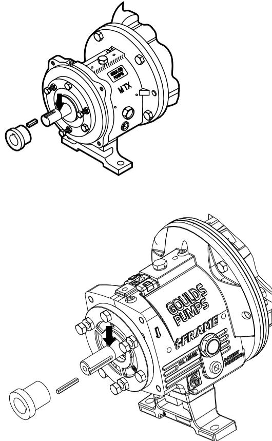
Figure 53: Coupling hub removal
