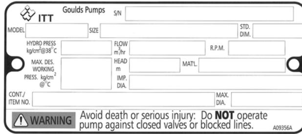
**Figure 14: Metric units - nameplate on pump casing**
