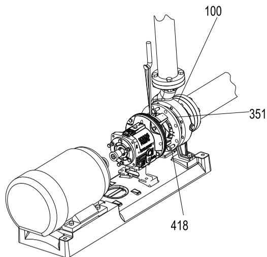
**Figure 134: Install back pull-out assembly**
