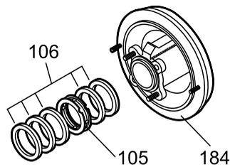
**Figure 62: Packing and lantern ring removal**
