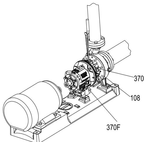
**Figure 136: Install and tighten casing jackscrews**
