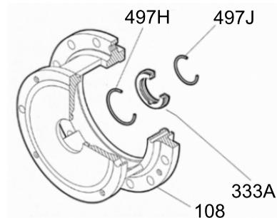
**Figure 65: O-ring removal**
