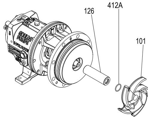
**Figure 128: Install shaft sleeve**
