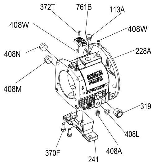
**Figure 104: Attach the bearing-frame foot**
