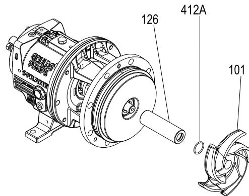
**Figure 125: Install shaft sleeve**
