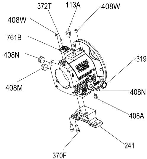
**Figure 99: Bearing frame foot reassembly**
