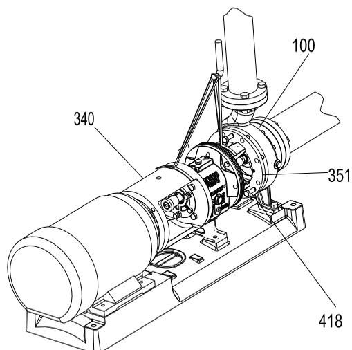
**Figure 52: Back pull-out assembly removal (without C-face adapter)**
