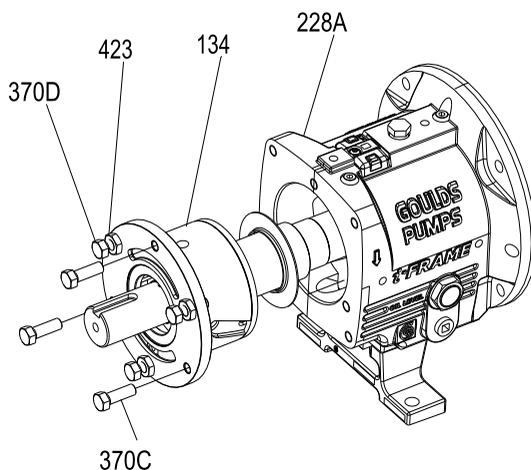
**Figure 75: Shaft assembly removal**
