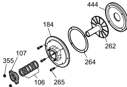
**Figure 64: Repeller removal**
