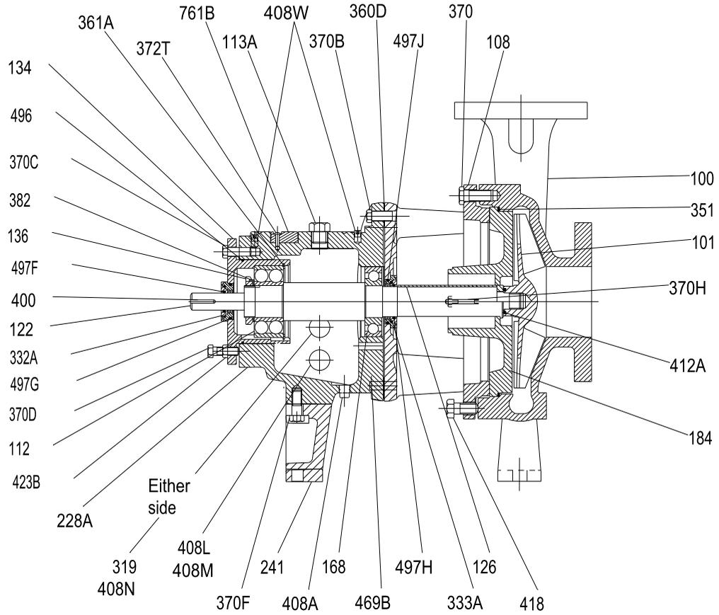
Figure 138: 3196 cross-sectional drawing
