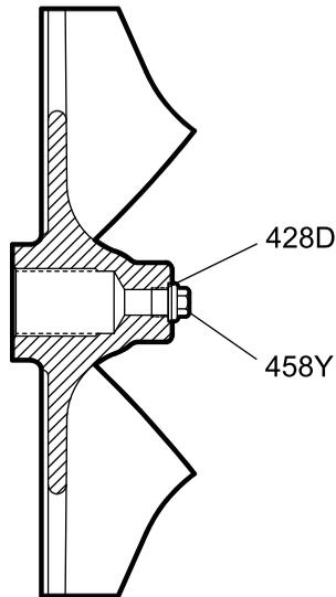
2. Spray penetrating oil through the plug hole into the cavity at the end of the shaft and let it penetrate for 15 minutes.
