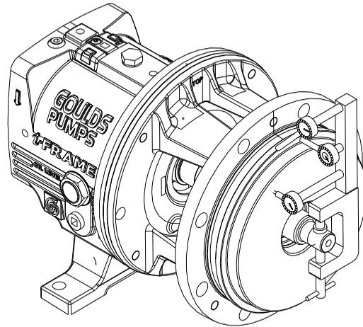
Figure 120: Checking for stuffing-box-cover runout
