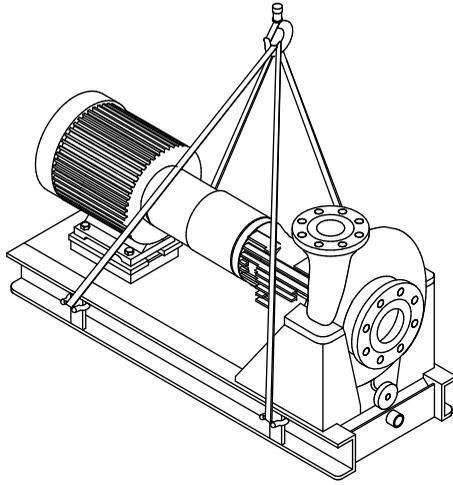
**Figure 4: Example of a proper lifting method**
