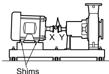
**Figure 27: Side view of an incorrect vertical alignment**
