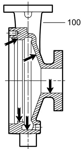
Figure 81: 3196, HT 3196, LF 3196, NM 3196, and 3198 casing
