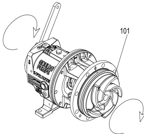
**Figure 129: Tighten the impeller**
