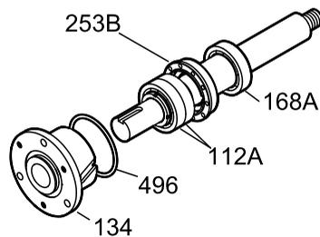
**Figure 77: Bearing housing and bearing removal**
