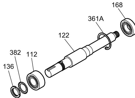
**Figure 96: Inboard bearing reassembly**
