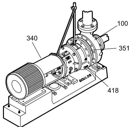
Figure 31: Example of the C-face adapter (340)
