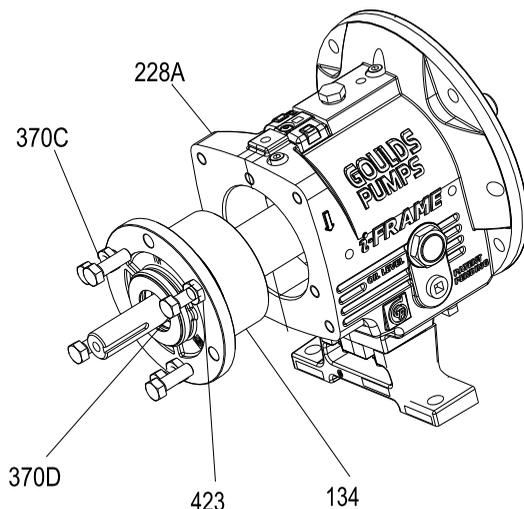
Figure 98: Jack bolt and locknut reassembly
