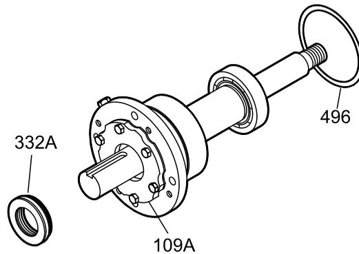
10. Install the shaft assembly into the bearing frame as follows (see the illustration):
