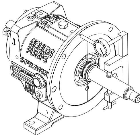
**Figure 113: Check frame-face run-out**
