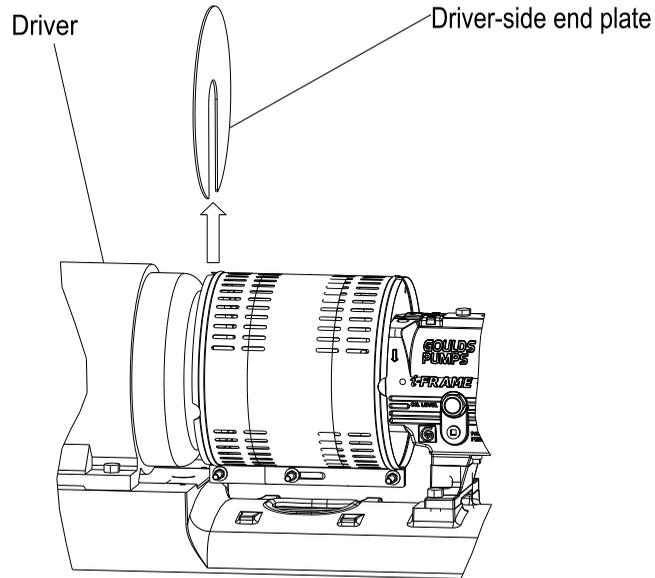
5. Remove the driver half of the coupling guard:
