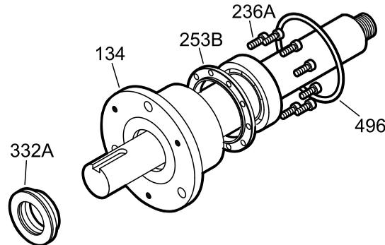
**Figure 103: Outboard labyrinth oil seal reassembly**
