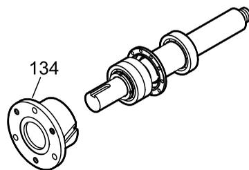
**Figure 107: Bearing housing reassembly**
