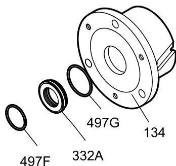
Figure 79: O-ring removal
