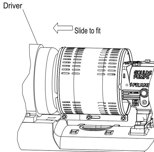
**Figure 43: Slide driver-half of coupling guard towards motor**
