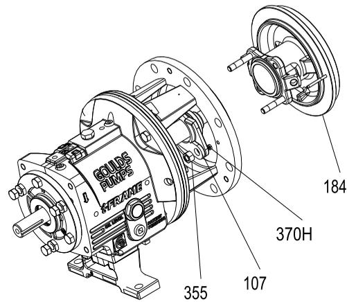
**Figure 60: Stuffing box cover removal**
