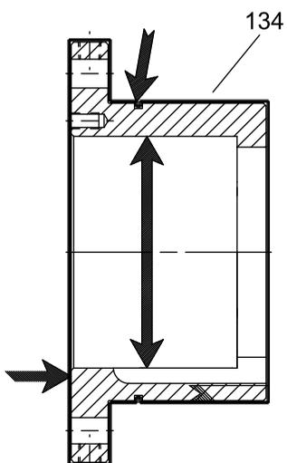
Figure 94: XLT-i and i17 bearing housing
