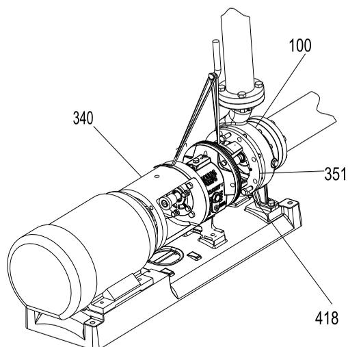
**Figure 135: Install back pull-out assembly**
