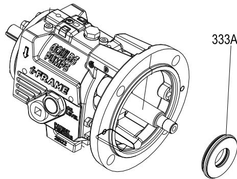
Figure 116: Position labyrinth oil-seal drain slots
