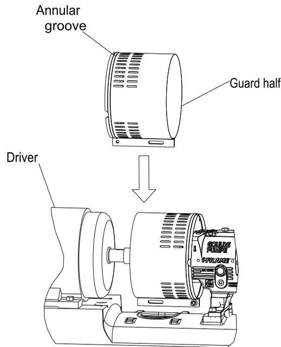
**Figure 41: Placement of driver half of coupling guard**
