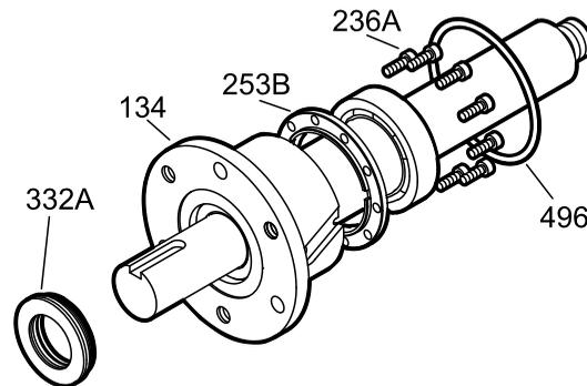
**Figure 108: Outboard labyrinth oil-seal reassembly**
