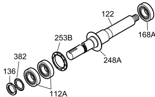
**Figure 106: Inboard bearing reassembly**
