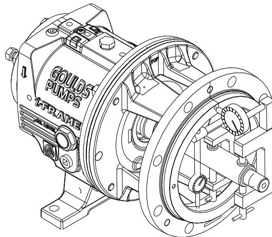
**Figure 115: Check adapter fit**
