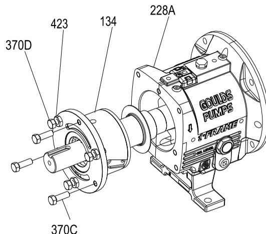
**Figure 109: Jack bolt and locknut installation**
