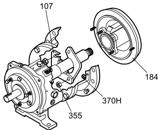
Figure 59: Stuffing box cover removal
