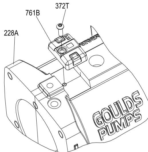
**Figure 132: Attach condition monitor to bearing frame**
