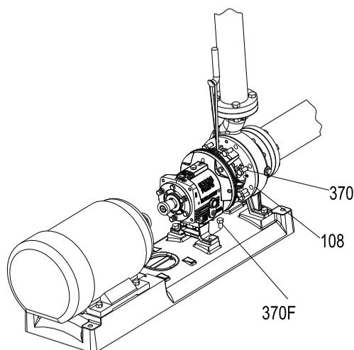
**Figure 51: Back pull-out assembly removal (with C-face adapter)**
