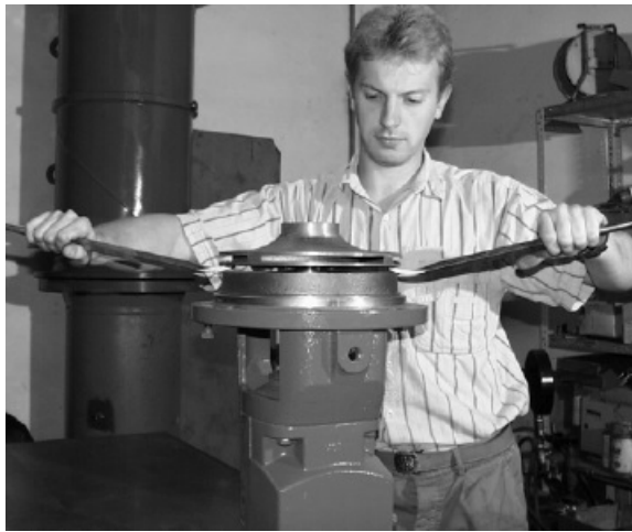
Figure 9: Place in vertical position to prevent tipping
