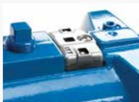
The heart of the i-FRAME®, the condition monitor unit continuously measures vibration and temperature at the thrust bearing and automatically indicates when pre-set levels
