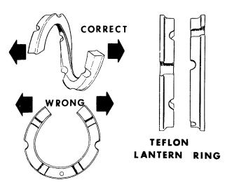
Group "L" pumps, staggering the joints. See sectional assembly, Section VI—C. Each ring should be firmly seated before the next ring is added. Two extra rings of packing are furnished in each set of packing. The extra ring for each side may be added as required.
