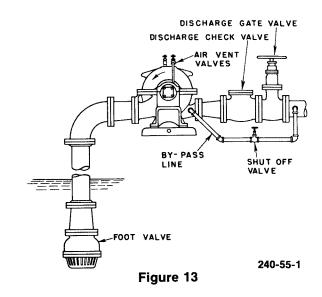
foot valve must be capable of withstanding static head pressure of the system.
