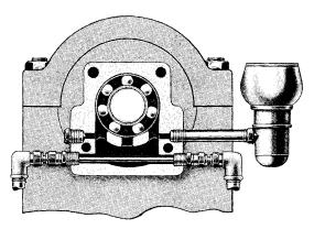
Water Cooled Bearing Construction
