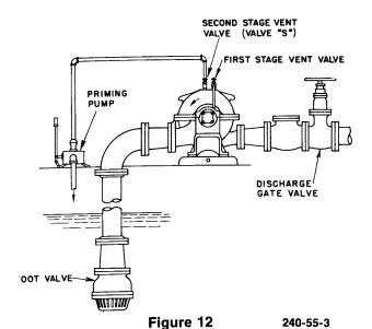
Close discharge gate valve (keep 1st stage air vent valves closed) and open 2nd stage air vent valve (valve "S") in line to priming pump. Exhaust air from pump and suction piping until water flows from priming pump. Close valve "S", start pump and open discharge gate valve.
