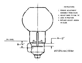
Fill the oiler bottle with oil, and replace in the oiler. The housing is filled when an oil level remains in the oiler bottle. More than one filling of the bottle may be required. Never fill the housing through the oiler without use of the
