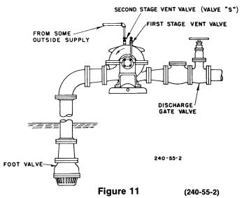
Close discharge gate valve, open 1st stage vent valve and open valve "S" in priming supply line until all air is expelled and water issues from vent opening. Close valve "S", close 1st stage air vent valve and start pump; then open discharge gate valve.
