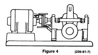
parallel but not concentric—by laying straight edge across both coupling rims at top, bot-
