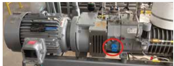
Figure 13: PD pump, side mounted to frame
