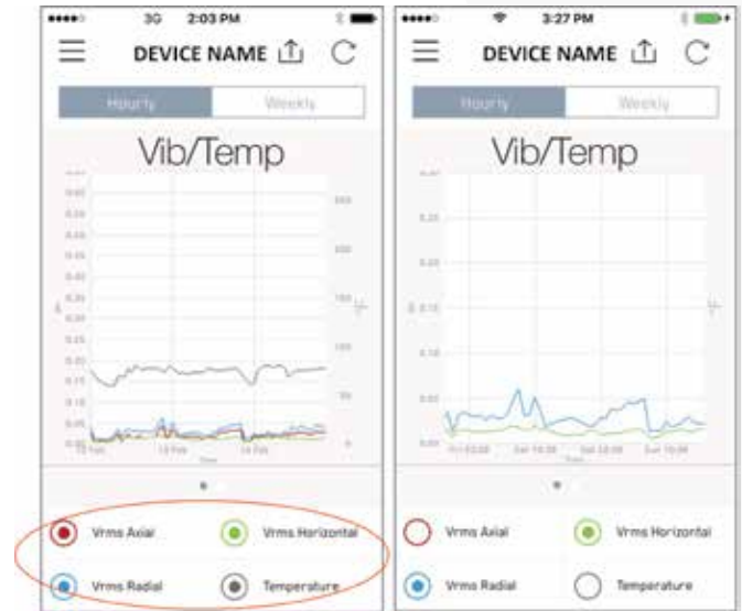
Figure 74: Default Trend view on left, trend view with several measurement de-selected shown on the right.
