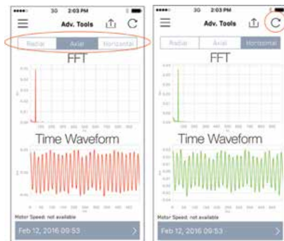
Figure 82: Switch between sensor axes or request updated dataset
