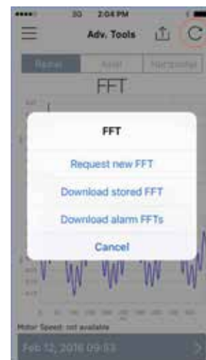
Figure 83: Request new FFT or access stored FFT datasets
