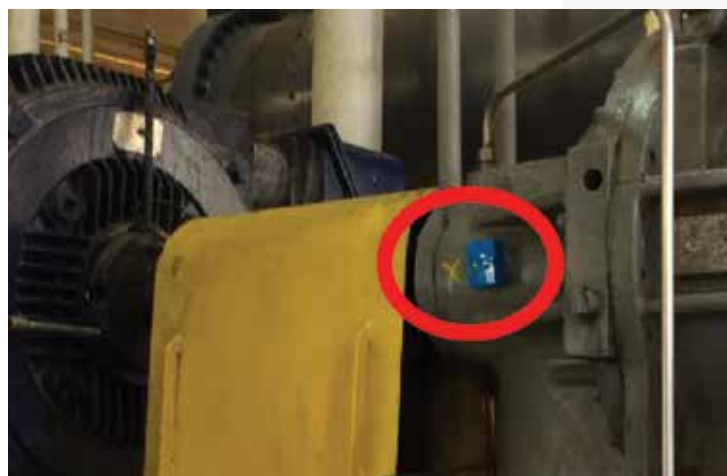
Figure 21: Vacuum Pump, side mounted to bearing housing
